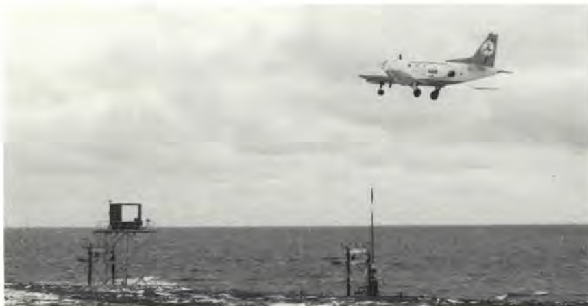
This is the Bendix MLS azimuth station at Shemya AFB, Alaska, during its FAA coming flight check. This particular antenna uses a 2-degree beam width.
