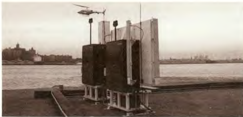
Locations that once were unsuitable for a precision approach can now have one thanks to MLS. A good example, is this Hazeltine Model 2500 located at the Wall Street, New York City Heliport. Photo courtesy of Hazeltine Corporation.
