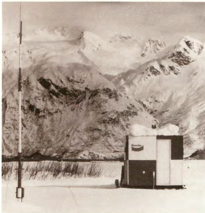
The MLS is capable of operating in mountainous terrain where ILS couldn't be used. It is also more reliable under adverse weather conditions. This MLS elevation station is located in Valdez, Alaska. Photo courtesy of Allied Bendix Aerospace.
